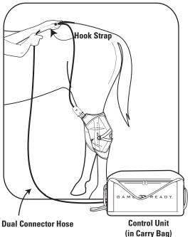
When using two Wraps simultaneously, use the Dual Connector Hose. Raise the Hose up and over the hindquarters of the horse to make a "Y" split. Connect each Hose to its corresponding Wrap. Adjust the length of the Hose by moving the Hook Strap up or down. Connect the single opposite end of the Connector Hose into the Control Unit.
