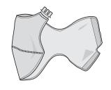
**fig. 3** Make sure the Heat Exchanger is flat inside the Sleeve with no folds or creases. Zip up the Sleeve. After assembly, fold at the natural vertical fold, and make sure the Wrap is flat and smooth.
