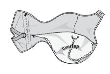
**fig. 2** Insert the Heat Exchanger into the Sleeve with the green side down. Slide the Connector through the opening in the Sleeve. The flaps of the Heat Exchanger must overlap slightly to fit into the Sleeve. The green side of the Heat Exchanger should touch the green side of the Sleeve.
