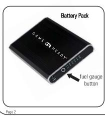
IMPORTANT- Activate the LED lights by pressing and holding the fuel gauge button for 20 seconds.
